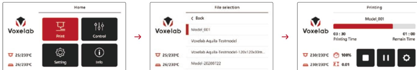
Note: When you notice the improper distance between the nozzle and the build plate during printing the first layer, please click the setting button to perform the z-axis offset.
